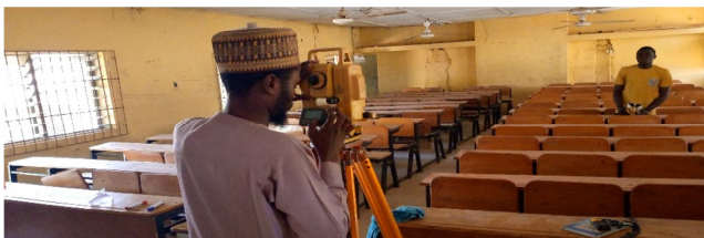
Figure 1. Location of Point in a Classroom Environment (Q/S Classroom) using NTS-350 infrared light total stations.
