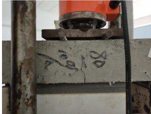
(a) Flexural - tensile test
