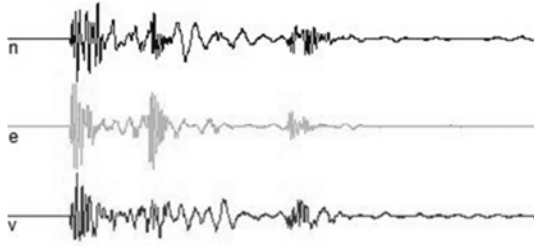
Figure 6. Typical three - component wave of blasting vibration.
