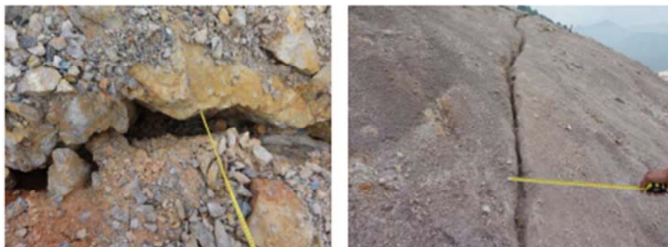
Figure 3. The extensional cracks on trailing edge.
