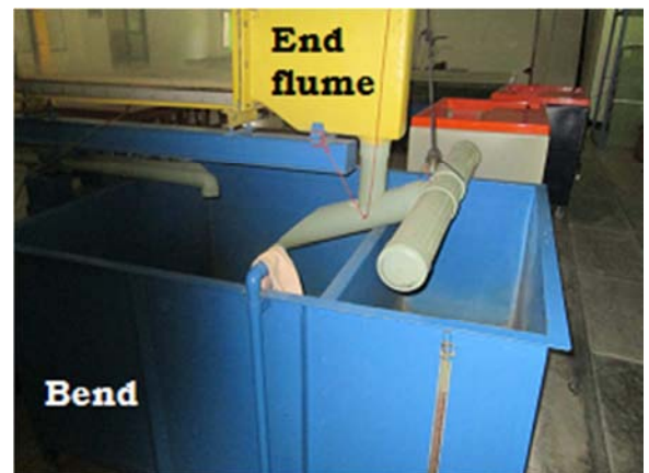
Figure 5. Bend for discharge measurement.
