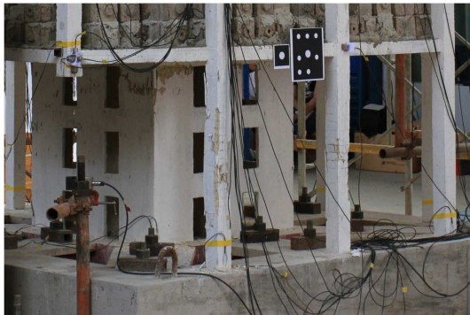
Figure 6. Damage of bottom structure under 7 th input at rare earthquake stage.
