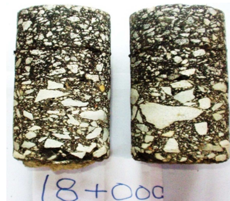
Figure 7. Asphalt cores with pitted surfaces.
