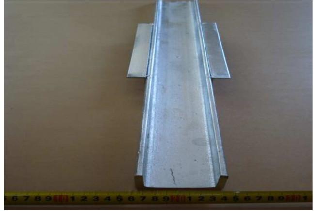
Fig. 2. Strip footing represented by steel channel.
