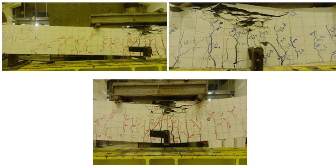
Figure 8. Pattern of Fractured of beams specimen use steel reinforced.
