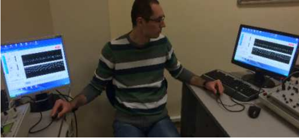
Figure 1. Simultaneous PPG signal recording from the left and the right index fingertips of a male volunteer.
