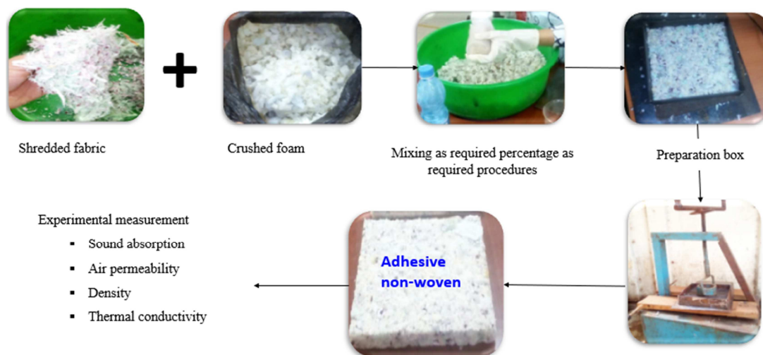
Figure 4. Development of adhesive bonded non-woven.
