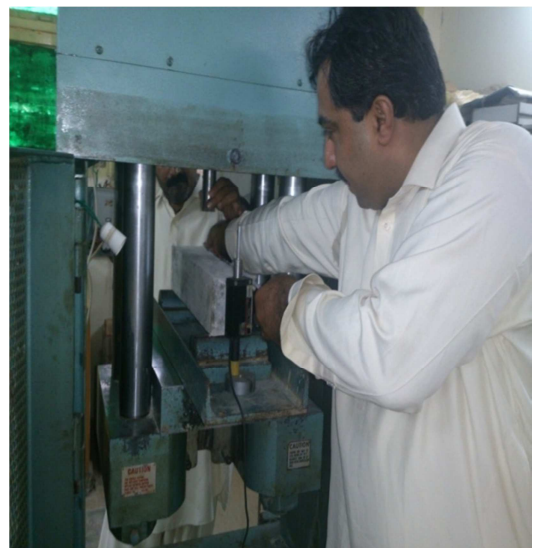
Figure 1. Adjustment of Beam in Testing Machine.
