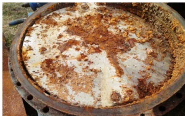
Figure 1. Biochemical corrosion, due to the deposits type crust combined with iron bacteria action on metal pipes.
