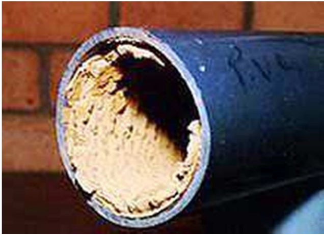
Figure 2. Biochemical corrosion due to the deposits crust type, combined with iron bacteria action in PVC pipes [9].
