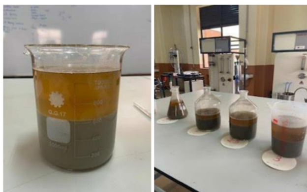
Figure 2. (a) dissolved salt and (b) decanted rock salt.
