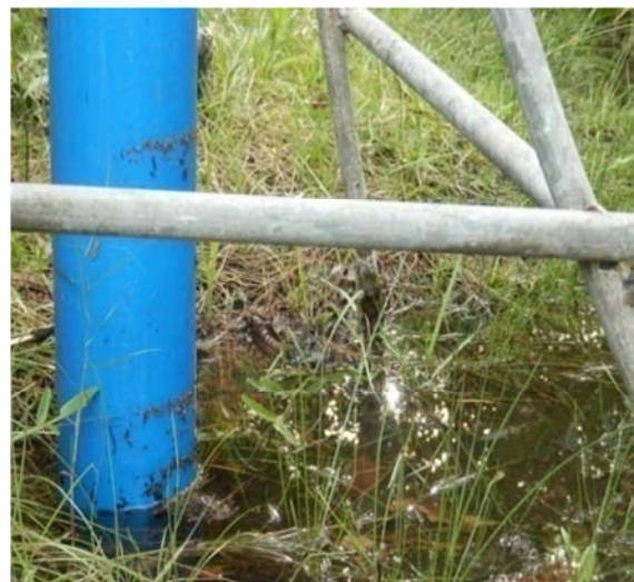
Figure 4. Signs of freshwater temporary floods followed by rapid fall of water levels at observation well 2 (OW2) on the South-end.
