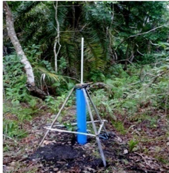
Figure 2. Water level recorder at South-end observation well 3.
