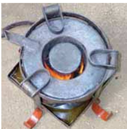
Figure 11b. Special, Kakute stove works by jatropha oil.
