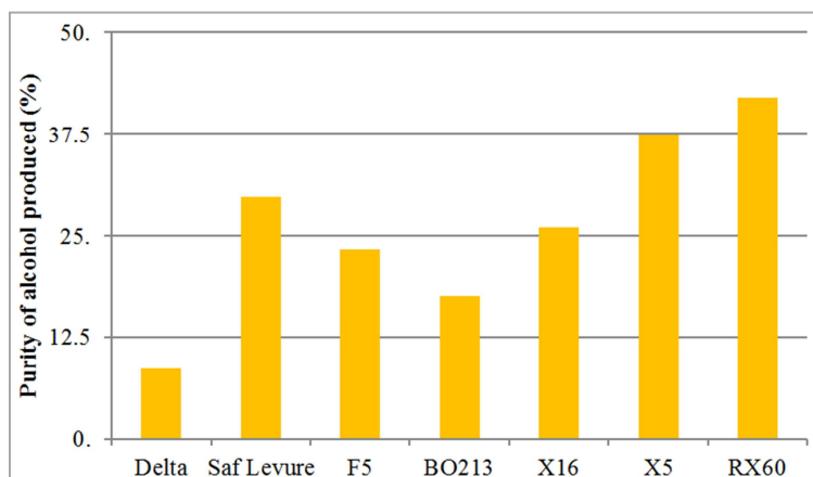
Figure 7. Purity of bioethanol produced according to the type of yeast used in the absence of urea.
