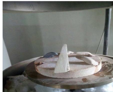
Figure 1. Pyrometric Cone Equivalent of Akure and Ile-Ife Anthill Clay.
