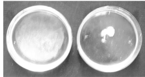
**Figure 8.** Left: the starch powder applied on the water surface with a potential of +250 mV forms a thin film that completely covers the water surface. Right: In the water with a potential of -200 mV, the powdered starch sinks [5].
