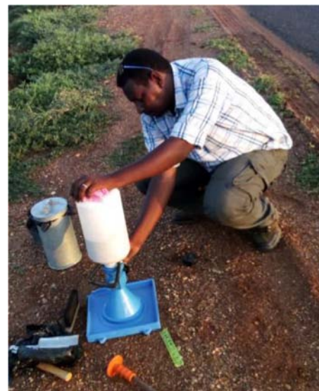
Figure 6. Field density test.
