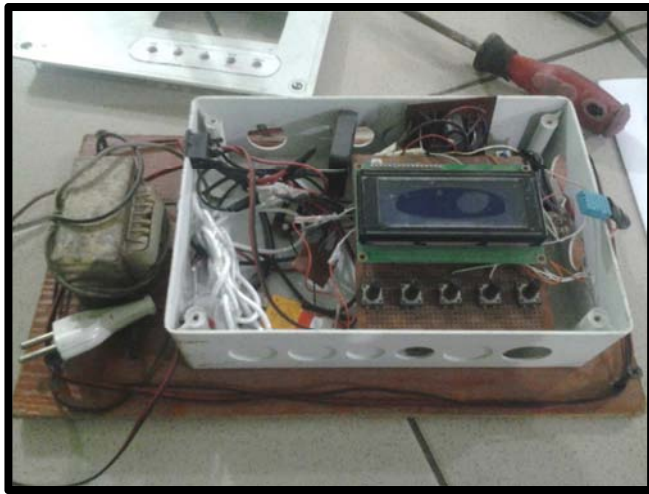
Figure 7. The developed weather instrument showing its display unit.
