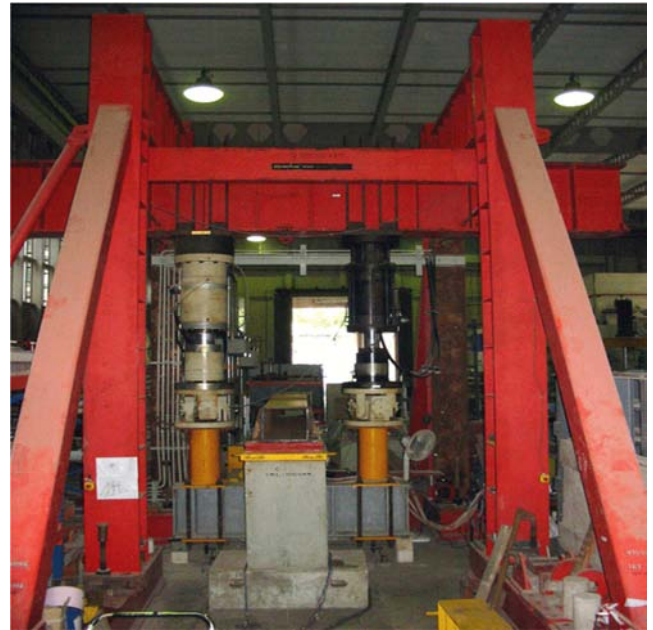
Figure 9. Test rig for SHS T-joint.
