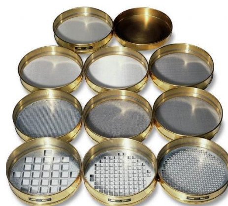
Figure 12. Shows sieve analysis.
