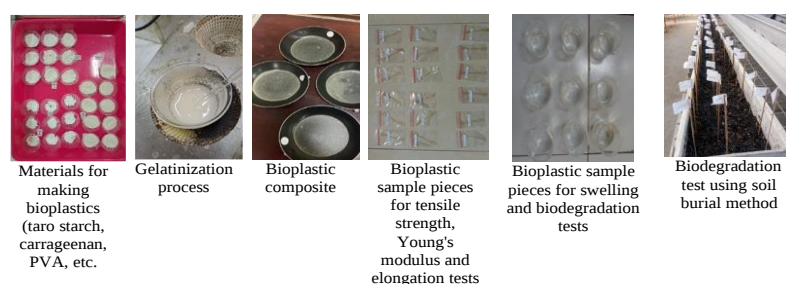
Figure 3. Preparation for testing such as tensile strength, elongation at break, elongation, swelling and biodegradation.
