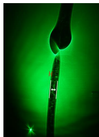
Figure 10. Shadow image of a human hair with a natural knot using a green laser pointer. Distance drop to wall: 2 m, total diameter: 12 cm \pm 70 \mu\text{m} (white bars). Medulla: 8 cm \pm 46 \mu\text{m} , distance to the cuticula 2 cm \pm 12 \mu\text{m} (red bars). The \pm sign is a standard deviation (SD).
