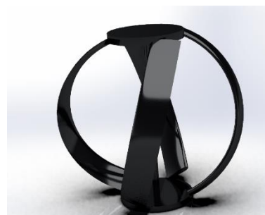
Figure 1. 3D modeled Gorlov pipe turbine geometry.
