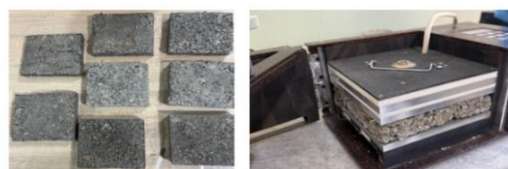
Figure 2. Thermal conductivity coefficient is determined using the ITS-1 device.
