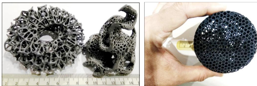
Figure 10. Skeletal polymer structures printed using the Multi Jet Fusion method.
