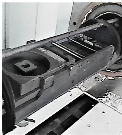
Figure 3. Appearance of the graphite unit of the device for forming an Al-Si layer from an Al melt.
