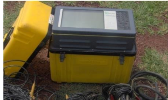
Figure 6. SmartSeis of Geotrix of USA for seismic refraction survey.
