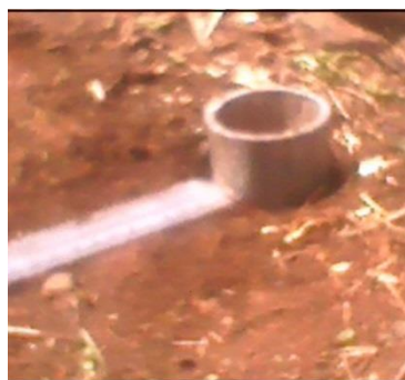
Figure 5. Photo after inserted 15cm soil depth the augur and 5cm leave above ground surface (hammered part).
