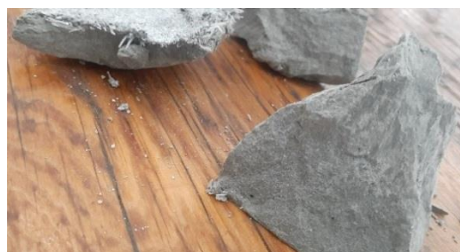
Figure 16. Uneven reinforcement in a set oil well cement specimen incorporated PET fibers.
