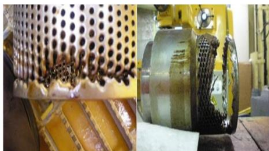
Figure 1. Problems caused by sand production in oil and gas wells: eroded sand limiting screen due to increased sand production rates [1].
