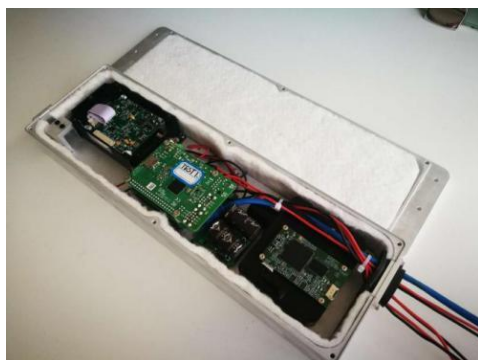
Figure 8. Structure of the Raman instrument within the protective enclosure.
