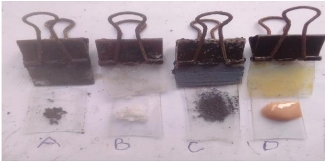
Figure 1. Samples and the thin films Carbon (A), CuAlSe 2 (B), Coal (C) and TiO 2 doped with RGO (D) TiO 2 on FTO glass substrate (solaronix).
