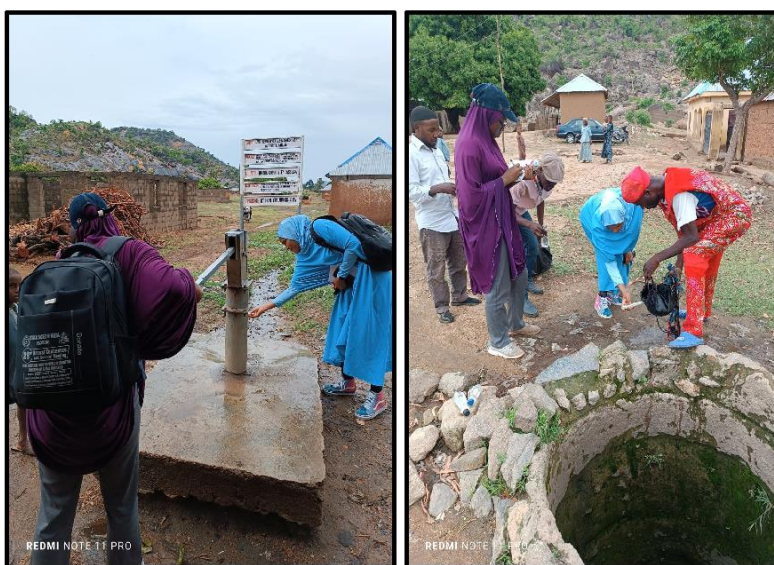
Figure 3. Field photograph showing analysis of physical parameters and water sample collection in open wells and boreholes.
