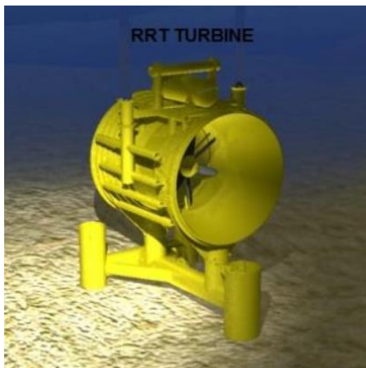
Figure 4. RRT turbine for dual kinetic acceleration nozzle.
