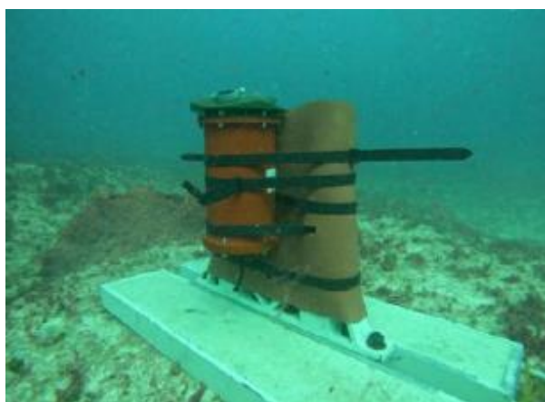
Figure 7. ADCP device installed at the bottom of the La Mona Channel at 64 feet of depth.
