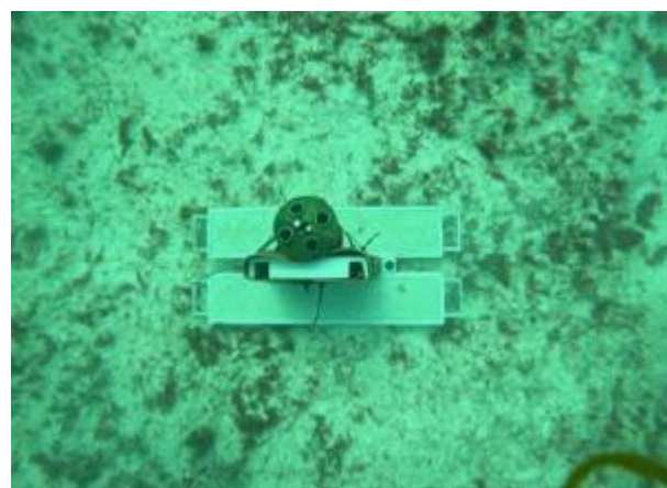
Figure 7. ADCP device installed at the bottom of the La Mona Channel at 64 feet of depth.
