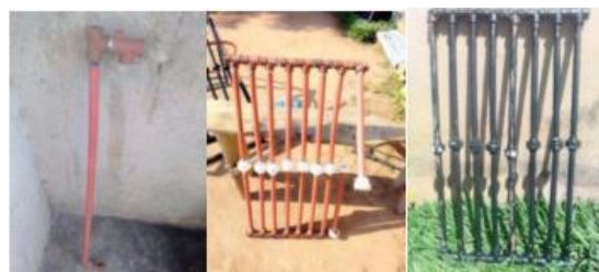
Figure 13. Connecting the pipes to the solar collector.
