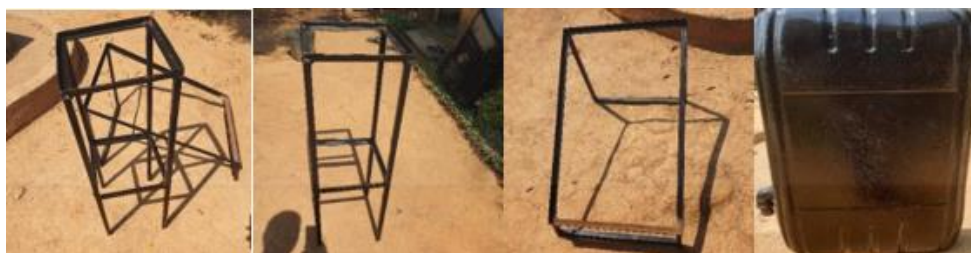
Figure 15. Solar collector and reservoir racks.
