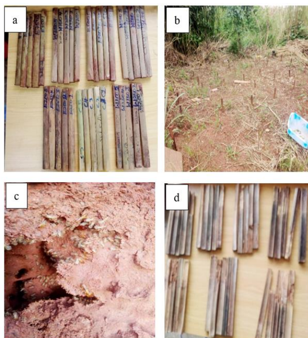
Figure 3. Field activities (a) Pre-exposure condition (b) In-ground field exposure (c) Subterranean termites (d) Post exposure condition of specimens.
