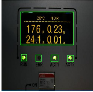
Figure 2. IPU Lamp Position and Screen Image Recognition.
