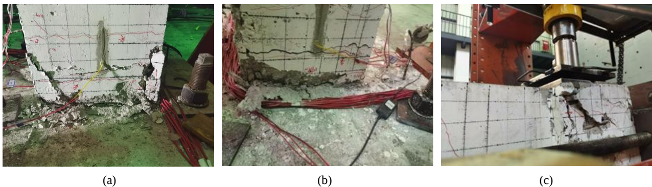
Figure 7. Crack patterns of specimen K1. (a) Low-ends of the left column, (b) Low-ends of the right column, (c) Beam-column joint.
