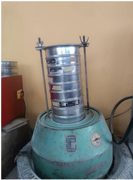
Figure 1. Set of British Standard sieves mounted on a mechanical shaker for particle size distribution analysis.
