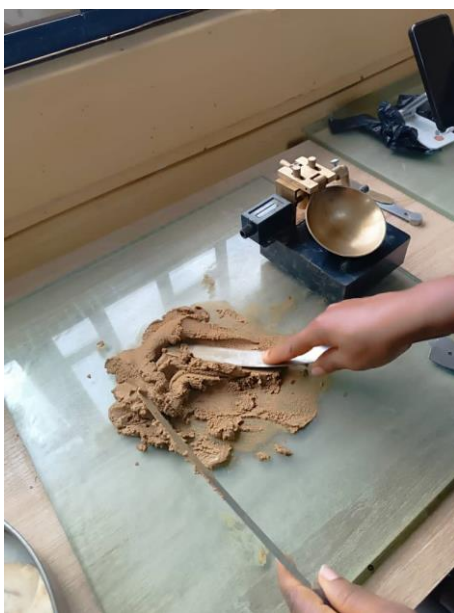
Figure 2. Casagrande apparatus setup for Atterberg limit testing, showing the liquid limit determination.
