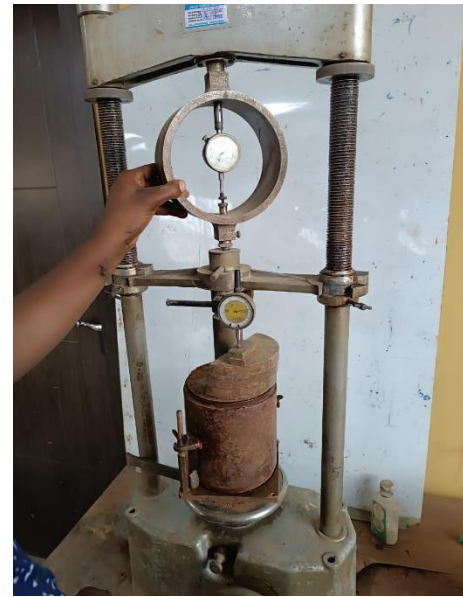
Figure 3. California Bearing Ratio (CBR) testing machine with loading frame and penetration piston.
