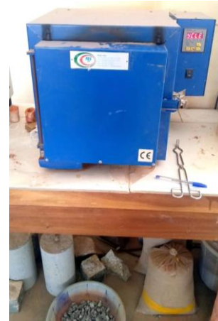
Figure 4. Calcination of CPHA.
