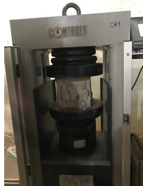
Figure 2. Experimental set-up for compressive strength testing.
