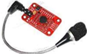
Figure 2. Microphone-fitted voice sensor.
