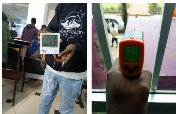
Figure 1. Dual Temperature Hygrometer smart sensor AR 867 (left) and Surface temperature thermometer (right).
