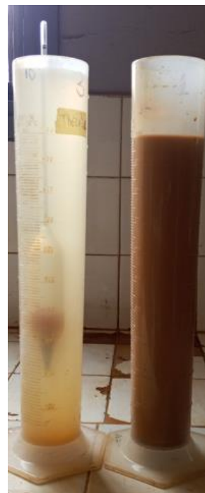
Figure 3. Sedimentation device used for particle size analysis of the fine fraction.
