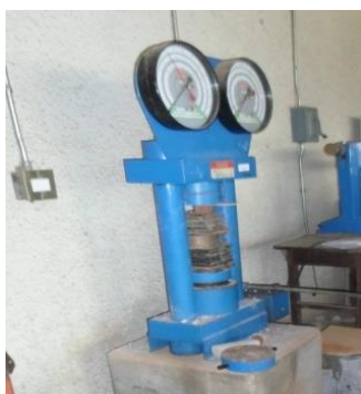
Figure 5. Compressive strength machine.
