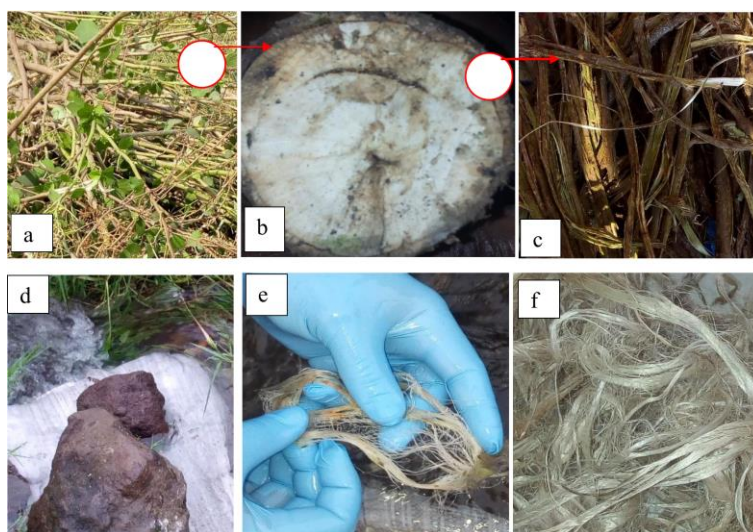
Figure 1. Illustration of the Urena Lobata fiber extraction process: (a) fresh UL stem, (b) UL stem cross-section, (c) UL stem bark, (d) UL fiber soaking, (e) UL fiber separation, and (f) UL fiber.
