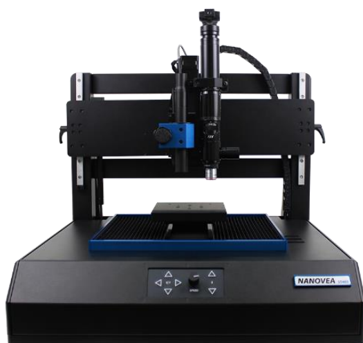
Figure 6. Surface profilometer machine to characterize the surface of the woven label print on the cloth. Our image is given.
