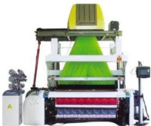
Figure 1. Woven label machines to print images on the woven label polymer cloth.
