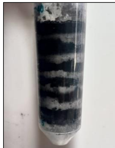
Figure 3. Adsorption column prepared using multilayer stacking of activated carbon and aluminium oxide.
